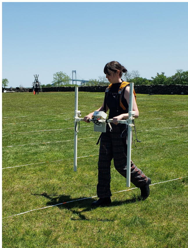
Salve Regina archeology students at work in the windmill field. Using Ground Penetrating Radar.
