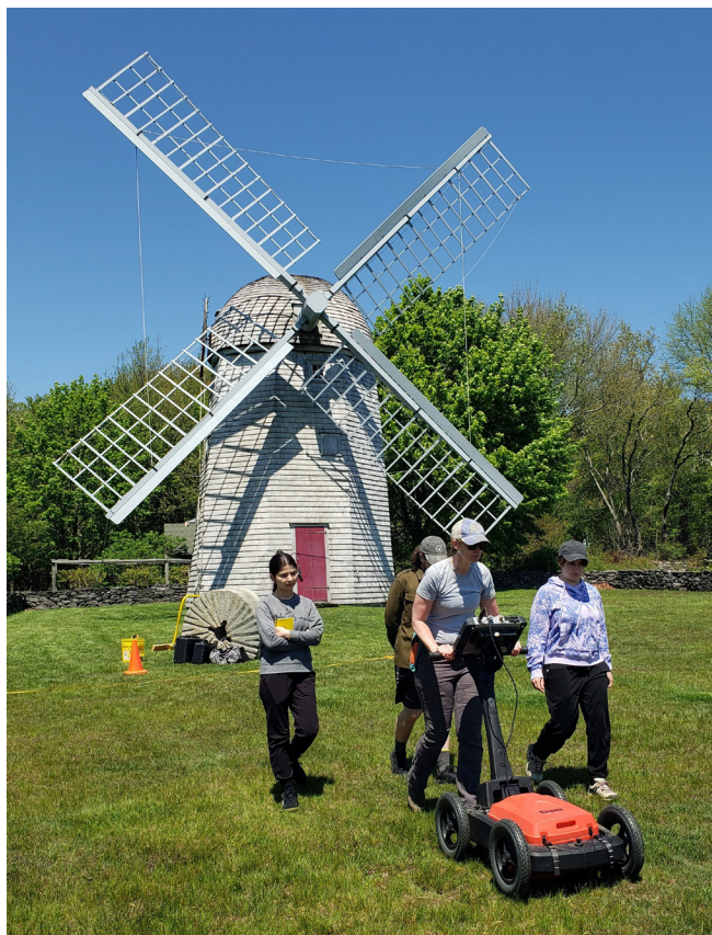
Salve Regina archeology students at work in the windmill field. Using Ground Penetrating Radar.
