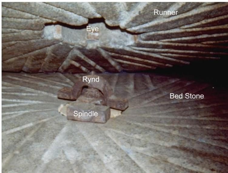
**tentering**, frees the stone so that it can rotate. The distance between the stones controls the quality of the meal that is ground – coarse for animal feed and fine for human use.
