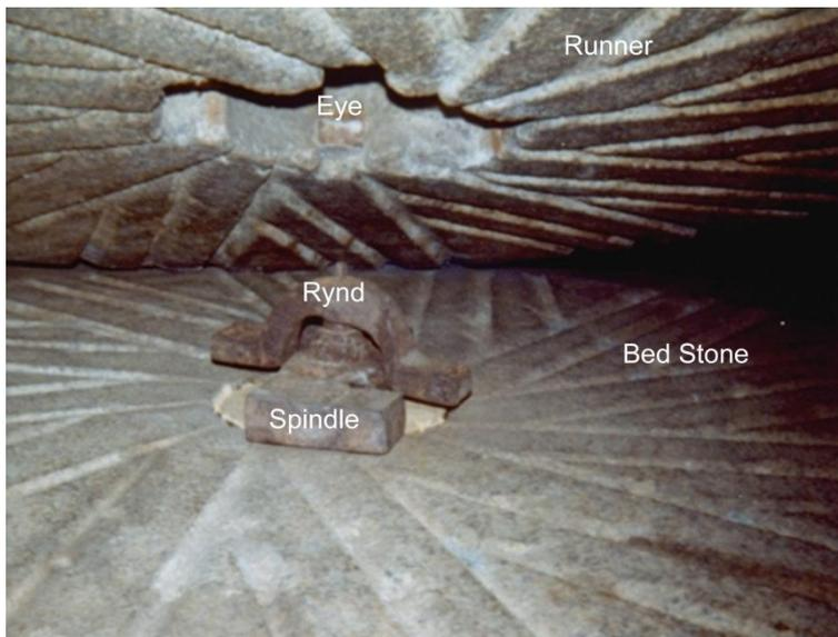
between the stones also controls the quality of the meal that is ground – coarse for animal feed and fine for human use.
